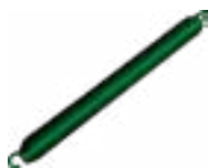
M-060MGREEN Spring wire Ø 5,2 mm, load 90 kg (green)
