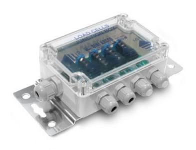
Junction box with 4 inputs and protection IP67 suitable for outdoor environments. It can be used as equalization or simple junction box of 2, 3 or 4 load cells. Screw terminal boards to facilitate the connection and signal adjustment trimmer, for an accurate and reliable equalization. The protection circuit protects from lightning and overvoltage.
