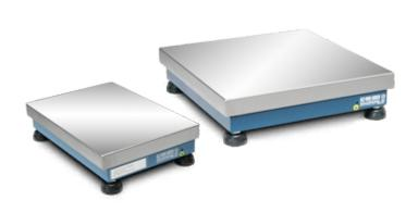
Small and medium capacity electronic platforms with a AISI304 stainless steel surface having a precise and sturdy structure, suitable for creating scales and automatic weight checking systems for all industrial and commercial applications. Standard version is with C6 6000 DIVISIONS approved load cell.
