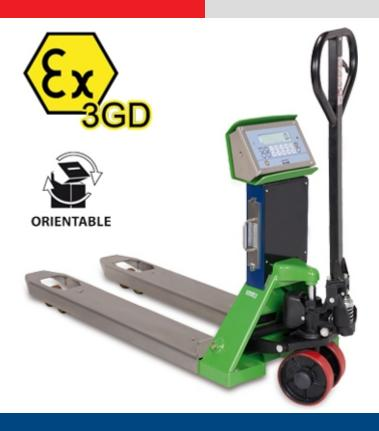
Pallet truck scales, with built-in electronic weighing, suitable for harsh working conditions and dangerous areas classified as hazardous (ZONE 2, 22) in accordance with Ex II 3GD IIC T6 T130°C X protection. The Atex certified four load cell weight detection guarantees the best accuracy in all work conditions.
