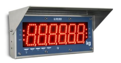
Weight indicator/ repeater with large matrix display composed of very intense bright LEDs. Particularly suitable for outdoor uses, it is clearly visible even in full sunlight and where it's necessary to view from a distance at any angle. Case completely in IP68 stainless steel. CE-M approved (OIML R-76 / EN 45501). MID approved (OIML R-61).
