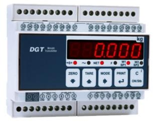
Multipurpose weight transmitter for panel mounting on DIN bar.**Ideal as an independent or dependent 4-channel digital junction box**, permitting the direct reading and diagnostics of each connected load cell. The wide range of available interfaces, makes it easy to integrate the weighing with any automation system. CE-M approvable (OIML R-76 / EN 45501).
